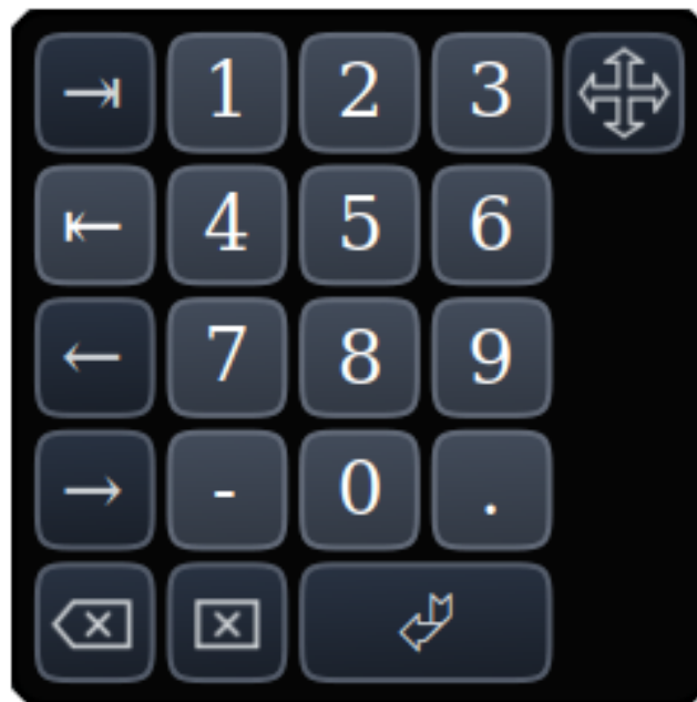
Figure 4.30: Number keypad - used for the CONVERSATIONAL Tab and the PARAMETERS Tab
